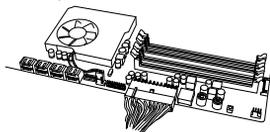
4. Connect the 4+4-pin EPS12V cable to the motherboard.
