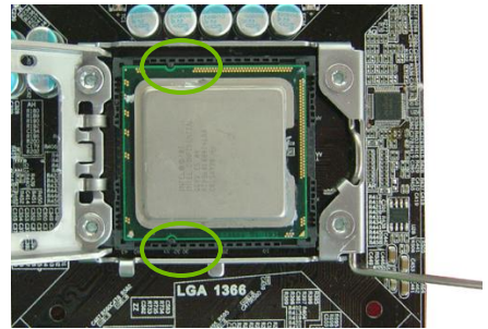
Align notches with notches on the CPU
