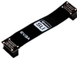
2Way SLI Bridge Link for attaching 2 graphics cards in SLI.
