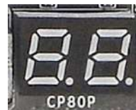
Debug LED with CPU Temperature Monitor
