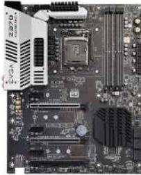
The EVGA Z370 Classified K Motherboard This motherboard contains the Intel® Z370 chipset.
