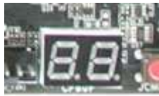
Debug LED with CPU Temperature Monitor
