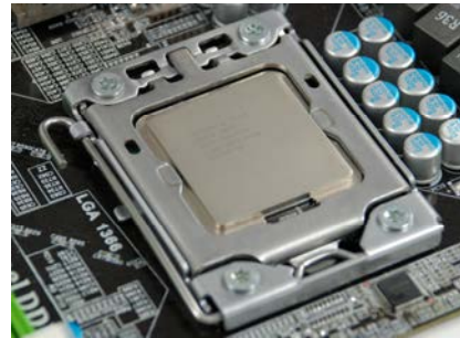
Align notches with notches on the CPU
