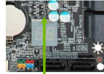
Debug LED with CPU Temperature Monitor
