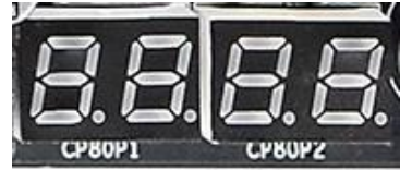
Debug LED with CPU Temperature Monitor
