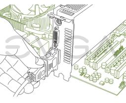
Insert your graphics card into either the PCI-E 2.0 slot or the PCI slot. The type of slot depends on the graphic card bus type. Connect a monitor to the output connector of the graphics card.
