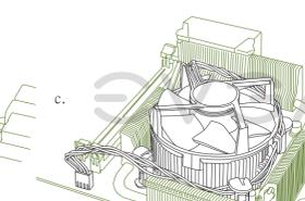
Apply a small, pea-sized drop of thermal paste on to the middle of the processor. Install your processor heatsink and fan.
