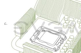
Unhook the socket lever and lift up the load plate. Remove the LGA 775 protective cover and carefully install your Intel processor making sure to properly align the notches. Close the load plate and with light pressure, lower the socket lever back in to its original position.
