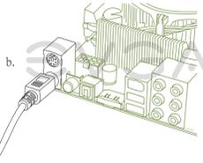
Plug in one keyboard into a USB port or PS/2 port.
