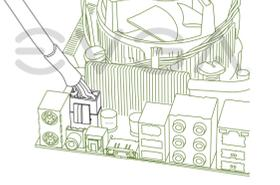
Make sure your power supply's power switch is in the OFF position then connect your 24-Pin ATX Power Connector and 8-Pin CPU Power Connector to the motherboard.
