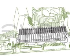
Install one stick of system memory (DIMM) in to the DIMM slot of your choice.
