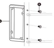
(2) Use 2x M3x10mm screws(C) to fasten the PSU Holder(D).
