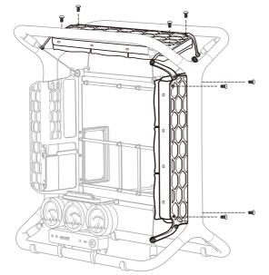
Fasten your radiator to an available mount location using the screws provided by your radiator or AlO device.
