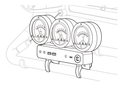
(1) With the clasp open, attach the Analog Gauge and front I/O to the E1 Carbon Fiber frame. (2) Once the module is in position, lift up the clasps to lock the module in place.
