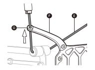
(2) Fasten M3x6mm screw(H) to fix the hook(F) and radiator mount.
