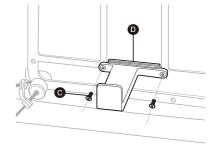
(3) Place your PSU on the PSU holder(D) and slide it into the PSU Bracket(A). Use the mounting screws provided with your PSU to fasten your PSU to the bracket(A)
