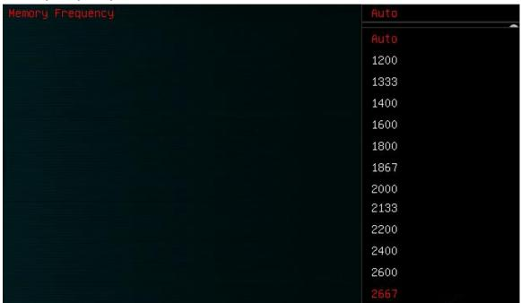
The memory controller can support memory speeds from 1200 through 2667 via multiplier adjustment. Anything above that will require BCLK adjustments.
