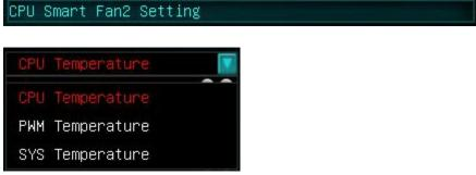
You can select what you want the curve to be based off of; once this is selected you have the same controls as CPU1. Keep in mind if you are using this for a secondary CPU fan, like for a push/pull setup, it is advised to use the same types of fans then set the Smart controls to be the same for CPU Fan1 and CPU Fan2.
