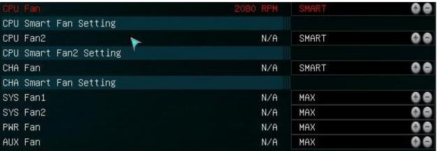
ALL FAN HEADERS ON THIS MOTHERBOARD HAVE A MAXIMUM POWER LIMIT OF 1 AMP @ 12 VOLTS, OR 12 WATTS, ANY MORE THAN THIS WILL LIKELY DAMAGE THE BOARD AND CAUSE PERMANENT FAILURE OF THE FAN HEADER. IF YOU NEED TO RUN A HIGH CAPACITY FAN, OR A PUMP THAT PULLS MORE THAN 1 AMP/12 WATTS, PLEASE USE A MOLEX CONNECTER FROM YOUR POWER SUPPLY, OR IF CONTROLLING THIS DEVICE IS NECESSARY, PLEASE LOOK TO A FAN CONTROLLER.
