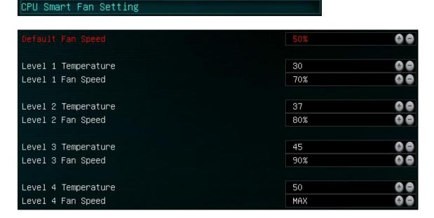
This is an example of a fairly aggressive fan curve, but not uncommon for overclocking or running in a warmer environment. At each Temperature Level you can manually enter any value in Celsius you want then below set what speed you want the fan to run at.
