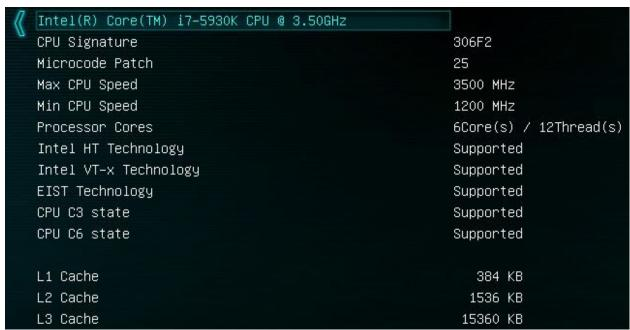
This section does not have any settings or adjustments whatsoever. This section provides a fairly in depth overview of the installed CPU, in the case of this test system, it is a 5930K, and it shows associated specs and what exactly it does and does not support.
