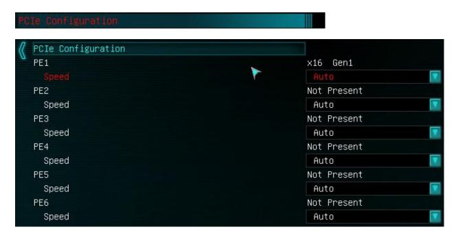
This option gives you as per slot breakdown showing how many lanes are being used by a given slot as well as what generation the PCIE device is running.
