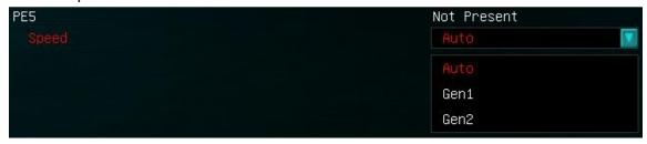
PE5 does \*NOT\* have an option for Gen3, as the lanes are not supplied from CPU but PCH which is limited to Gen2.
