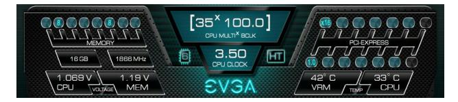
In the center above the EVGA logo, is basic CPU information. There is the overall CPU clock speed shown in GHz (Gigahertz). Above that the CPU Multiplier times Base Clock (BCLK) which is how clock speed is derived. Adjacent to the CPU Clock there is a small outline of a chip and a number inside of it, the number in this case 6, is the number of physical cores in the CPU. HT indicates that Hyper Threading is enabled.
