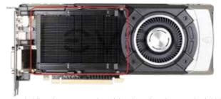
6) Remove the 4 screws holding the center portion of the shroud, and remove it. (#000 Philips bit)
