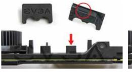
11) Remove the plastic cap on water block, use the 4 Spring Screws previously removed to mount the block on the GPU (Thermal compound is pre-applied to the block).
