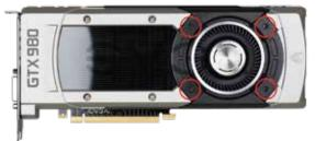
14) Attach the shroud to the card, you can use the hoses and the fan as alignment marks. It will use the
