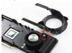
9) Be sure to clean the GPU (see pic) with alcohol (preferably 90%) removing all thermal compound.
