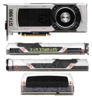
3) Remove the 4 spring screws on the back side of the card (#1 Phillips Bit) this will allow the heatsink to be removed.
