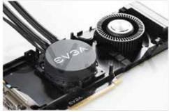
cards power header, then reattach the fan to the card via the pass through. Make sure the wires do not touch the fan; please use included strips of tape to attach the wires to the plastic around
