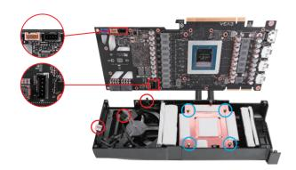
6. Remove the GPU/Memory baseplate from the HYBRID kit and place it over the 4 mounting holes over the pump/waterblock as seen in the image below. At this time, remove any protective covering/tape over the thermal pads before moving to the next step.
