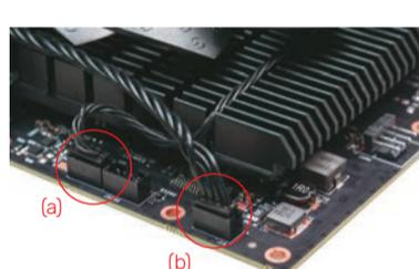
9. Position the shroud adjacent to the graphics card by using the tubes as a reference. Carefully connect the RGB LED connector on the shroud to the RGB header, circled in the image below. Take care that the cables remain away from the fan.
