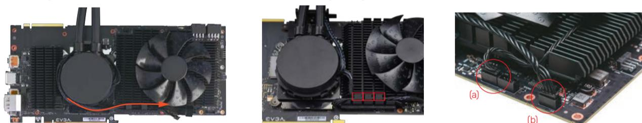
9. Position the shroud adjacent to the graphics card by using the tubes as a reference. Carefully connect the RGB LED connector on the shroud to the RGB header, circled in the image below. Take care that the cables remain away from the fan.
