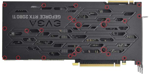
2. Remove the screws circled on the bracket in the image to the right with a Phillips #1 screwdriver and remove the bracket. Carefully set 4 screws aside, as you will need them later. The #15 2 Slot bracket will be installed at Step 11.
