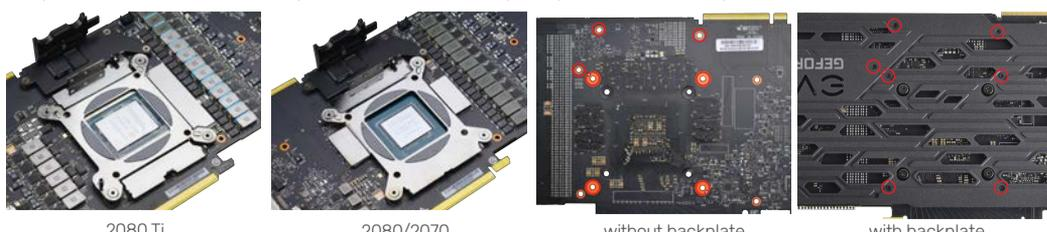
6. Install the VRM Heatsink. Remove the protective tape on the bottom of the heatsink(s).
