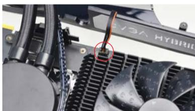
10. Install HYBRID radiator fan cable and the shroud
