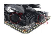
9. Position the shroud adjacent to the graphics card by using the tubes as a reference. Carefully connect the RGB LED connector on the shroud to the RGB connector that runs through the VRM heatsink. Take care that the cables remain away from the fan.
