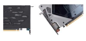
At this point, your waterblock should be fully tightened and ready to test. As noted before, please use care to avoid overtightening, as this may strip the screws and/or damage the graphics card. Lastly, do not use power tools to install the waterblock or backplate.
