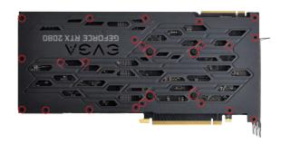
2. Remove the screws circled on the bracket to the right with a Phillips #1 screwdriver and set the screws aside, You will need to reinstall some screws after installation of the waterblock.
