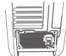
3. Use the screws provided with your case to install the power supply into your computer. **NOTE:** It is recommended to install the power supply with the fan facing down. However, if your case places the power supply at the bottom of the case and there are no ventilation holes available, it may be best to install the power supply with the fan facing up for greater efficiency and reliability.
