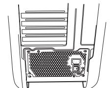
3. Use the screws provided with your case to install the power supply into your computer. **NOTE:** It is recommended to install the power supply with the fan facing down. However, if your case places the power supply at the bottom of the case and there are no ventilation holes available, it may be best to install the power supply with the fan facing up for greater efficiency and reliability.
