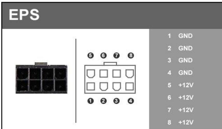
**EPS PWR 8P**, the 8-pin ATX 12V power connection(s), is used to provide power to the CPU. Align the pins to the connector and press firmly until seated. Additional EPS, if present, is optional for improved overclocking. Please remember to make sure that the tab on the EPS socket is aligned with the release clip on the cable.
