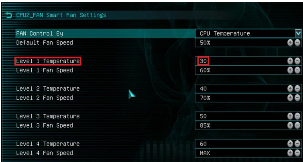
There are four tiers of temp control, with Level 4 fan speeds generally recommended to be set at Max. The example above uses a fairly aggressive fan curve, but you can set this as high or low as you wish. Make sure, however, to stay below 5-10C of the Max safe load temp for your specific processor, which can be found at [Ark.Intel.com](http://Ark.Intel.com). All Smart Fan Settings have the same controls and can be setup the same way.
