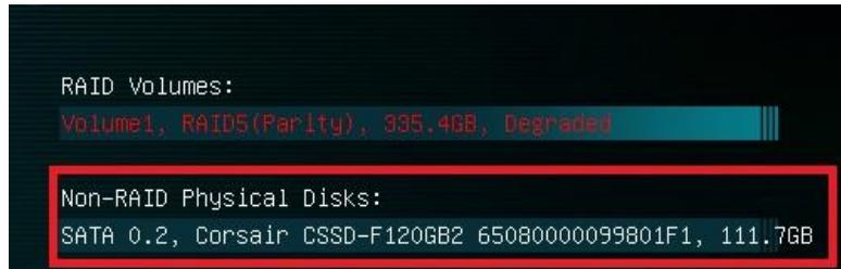
Select the degraded RAID volume, then select “Rebuild” on the following menu.
