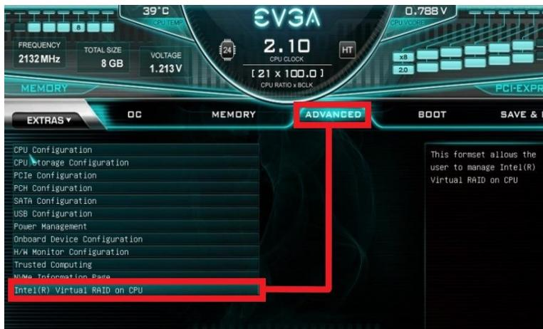
Once in the Intel® Virtual RAID on CPU menu, you can create your RAID array. The steps are similar to creating a RAID array through either the SATA or sSATA controller, which can be found on Pages 72-74.
