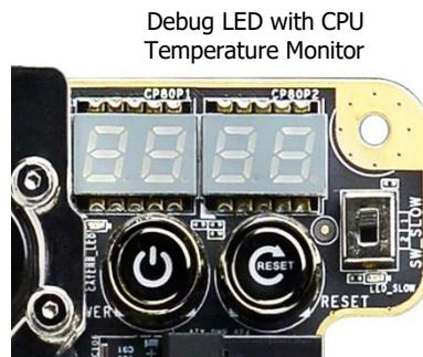
This Debug LED will switch to display the user's 80Port Configuration settings after POST (see Page 149). Please note that if you see the Debug LED constantly switching numbers after entering Windows, the Debug LED is showing temperature or voltage information, and is NOT reporting errors.
