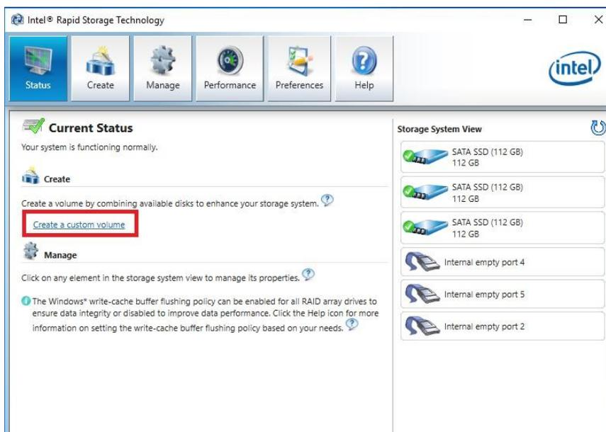
This guide will illustrate how to create a RAID1 array using the IRST. Using the screen above, we know that three (3) SSDs are currently attached to the controller and the other three (3) INTEL® SATA ports are empty (this can vary board to board based on how many Intel® SATA ports are present). If you plan to create another type of array, please ensure that you have the correct number of drives attached and shown on the status screen in IRST for your intended array before you start.
