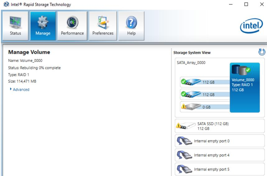
The rebuild process will begin. As with any RAID array with Fault Tolerance, the rebuilding time depends on several factors, such as array size, array type, CPU, etc. You will then see the Rebuild % status in the Manage tab. Once repairs are complete, the array will update to “Status: Normal.”
