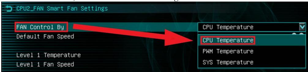
First, choose the temperature monitor the PWM controller will use to monitor for its temp information. It's recommended to link the fan control to the CPU, which is predominantly the most important temperature in the system. The exception is when you have 32GB of heavily overclocked RAM, which may cause PWM temps to be a concern. If this is a concern, set the fan control to the PWM temp.
