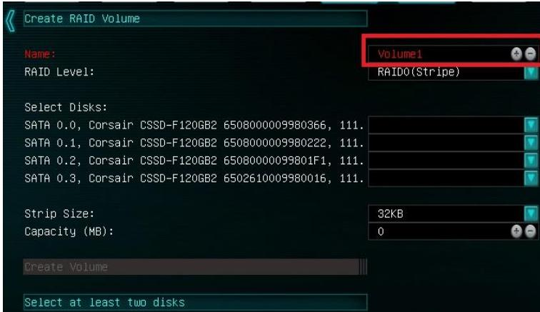
Next, select your intended array type. This can be done by either clicking on the down arrow and clicking on the RAID level you want, or pressing the enter key and using the down arrow to select the RAID level and pressing Enter again. Please see the top half of Page 70 for a quick reference on different RAID levels and RAID types based on your total number of drives.
