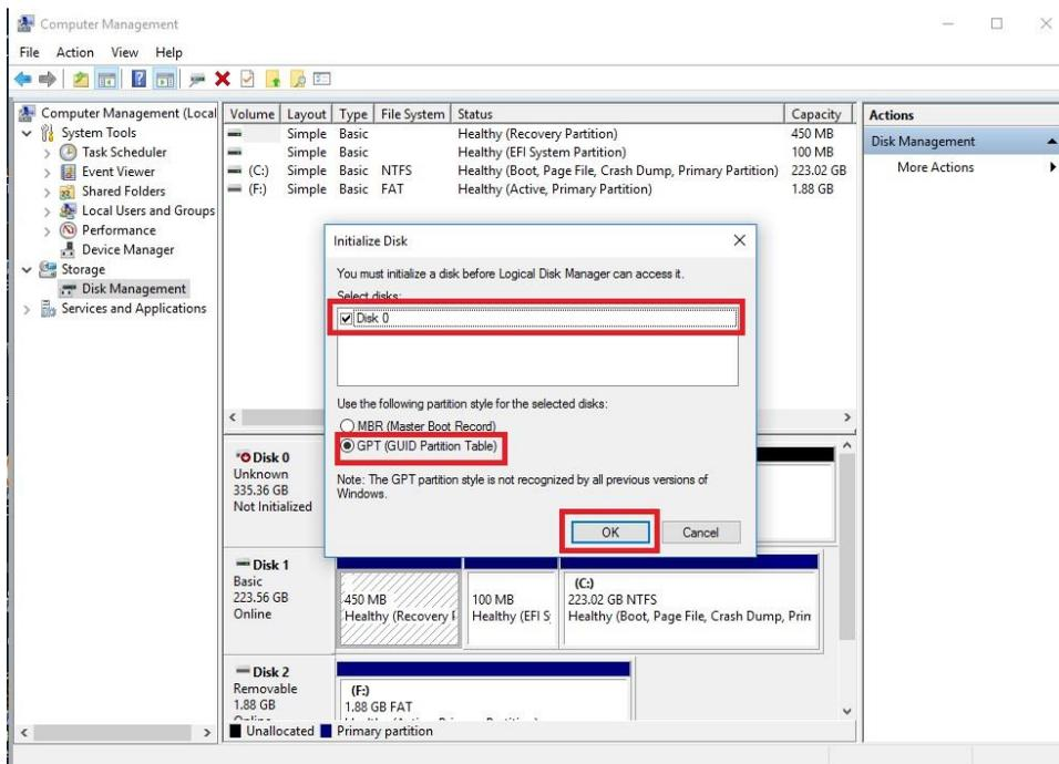
Before you can assign a drive letter to a drive or array, the initialized disk must be partitioned. If you are following this guide and just initialized your drive or array, the New Simple Volume Wizard will automatically pop-up.
