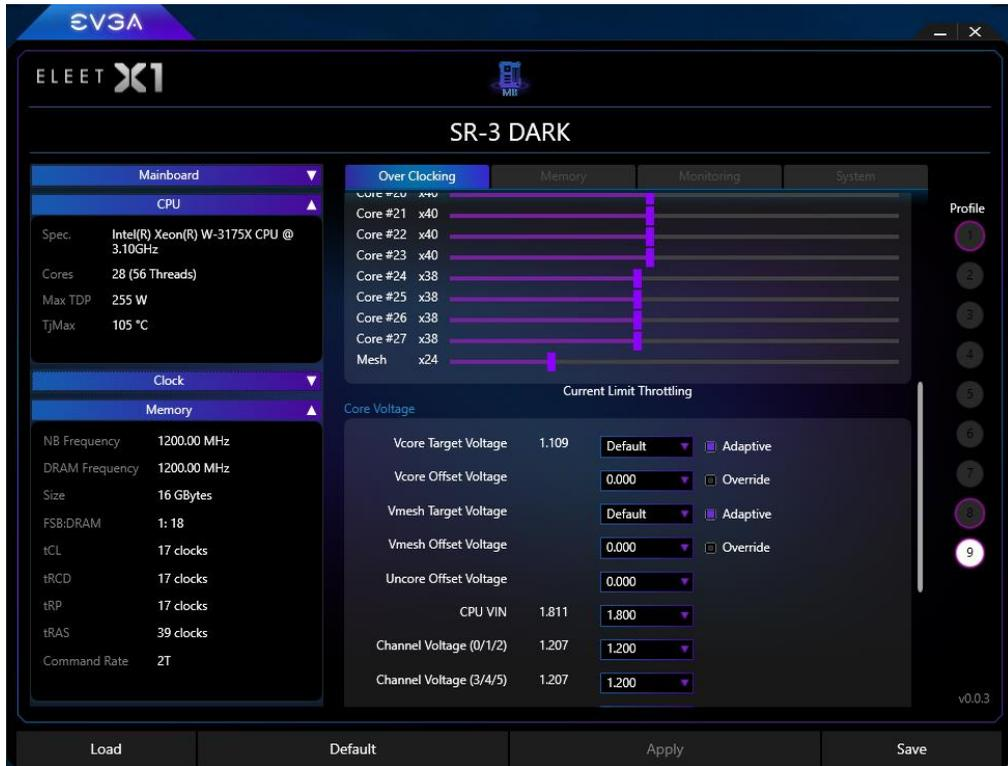
As seen above, there are options for multiple voltages, and two options for your CPU Vcore and Vmesh: Adaptive and Override voltages. Adaptive allows for a tighter voltage profile to keep voltage and heat to a minimum, while Override is more of a brute-force method of setting your voltage. One primary advantage of using a stable Adaptive voltage is that it allows your CPU to properly take advantage of C-States and energy saving features, which can extend the lifespan of your CPU.
