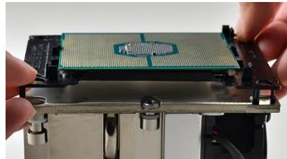
3. When properly installed, the CPU and clip will be fully inserted in each mounting hole and the clip will be flush against the CPU cooler.
