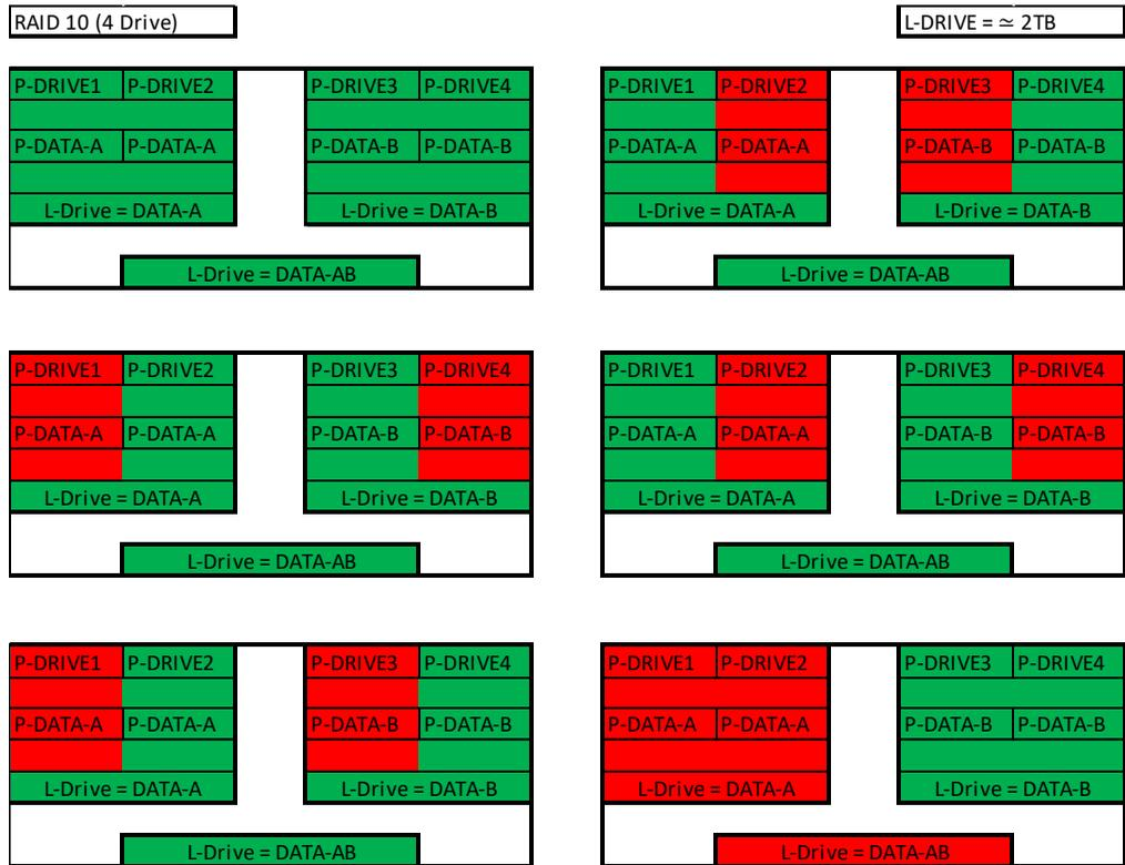
While the SR-3 DARK controller will support a four drive RAID10 array, RAID10 can scale indefinitely provided the controller supports more drives. Every pair of drives adds an additional mirrored node, which increases the theoretical number of failures the array can suffer before a loss of data occurs. However, an array can still fail due to both drives on a node failing.
