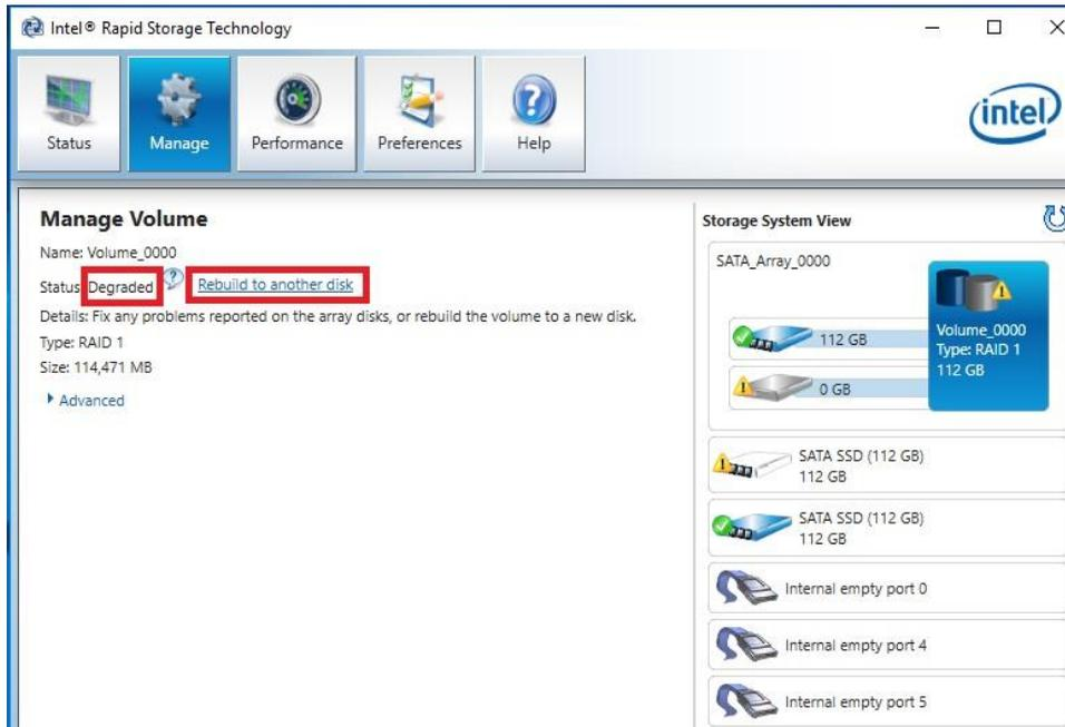
Next to “Status: Degraded,” left-click the hyperlink labeled “Rebuild to another disk.” This will bring a pop-up window over the IRST showing a list of attached drives that can be used for the repair (see pic on next page):
