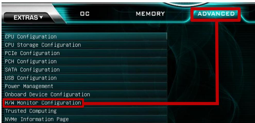
Once into the H/W Monitor section, you can see the temperature monitors across the top. Below the monitors, each fan is already configured in Smart mode, which means the fan controller is using a Smart curve for fan controls. Each fan can be set to a separate fan curve. To set a Smart curve, please see the guide starting at the top of the next page.
