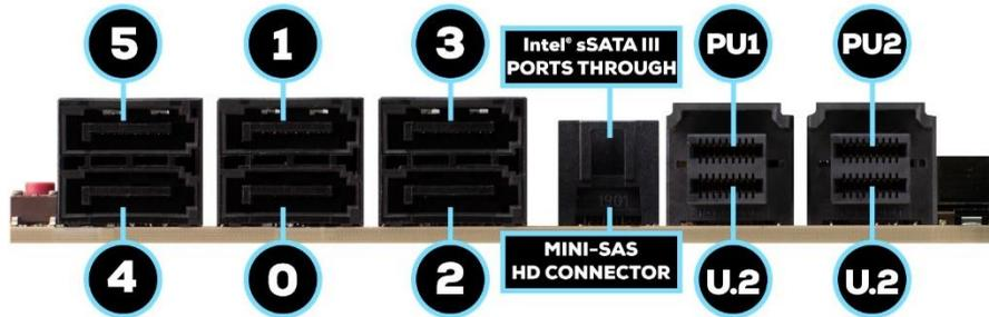
SATA ports on this platform natively support full AHCI and RAID functions. AHCI is enabled by default, but the controller can be put into RAID mode in the BIOS. RAID mode supports RAID levels 0, 1, 5, and 10 through the Intel® controller. RAID-ready ports also have full AHCI functionality.
