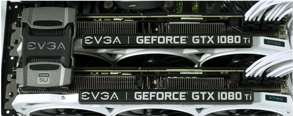
2. After the cards are installed, have power connected, and the SLI/NVLink bridge is attached, boot into Windows. The graphics driver will normally identify the cards and automatically configure the driver. If not, then you may need to reinstall the driver.
