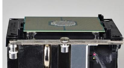
You are now ready to install the CPU to the motherboard. Remove the cover from the CPU socket if you have not already done so.
