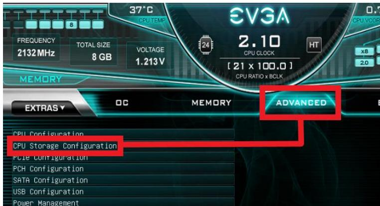
Inside the CPU Storage Configuration, each VMD slot/port will be listed. Click the dropdown box for each installed VMD device and select “PCIe SSD Card” to both enable the Intel® Virtual RAID on CPU menu, and to make the device visible later when you select your devices for your RAID:
