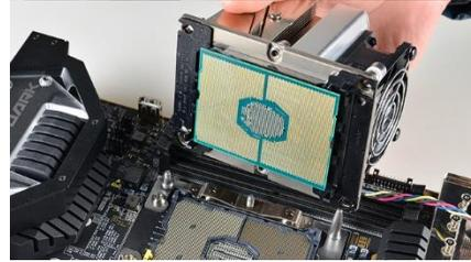
**Note:** The gold triangle key on the CPU should match the triangle key on the load plate.
