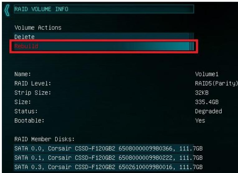
Next, you will see a list of all attached HDD/SSDs that can be used to rebuild the array. Select the disk, then click on it or press enter.
