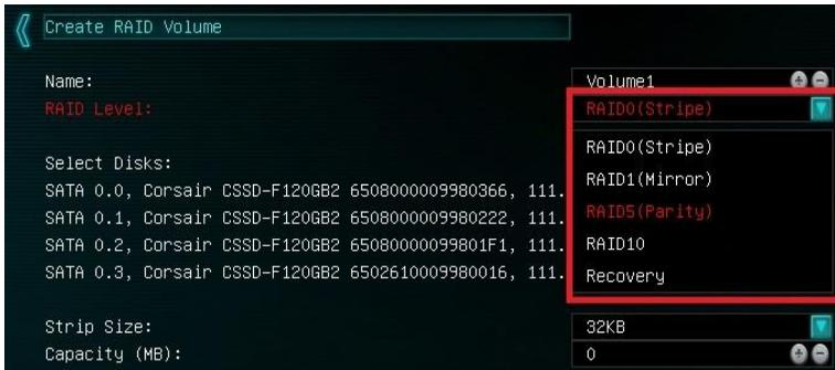
Next, select the drives you want to use for the array. Select the down arrow and the “X” for each drive you want to include in the array.
