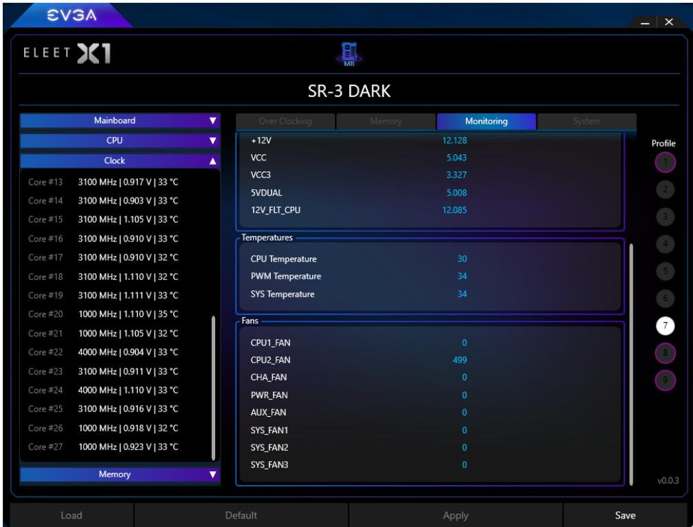
The Monitoring page only supports a static readout of each voltage, temperature, and fan speed. Settings cannot be adjusted or manipulated on this page.
