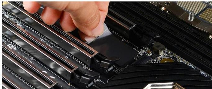
3. Insert the M.2 device at a slight angle of approximately 45 degrees to the board. This will allow the contacts (colloquially called “Gold Fingers”) to seat completely into the slot. If the device is fully seated, you should be able to release it and the device will rest at an angle of about 30 degrees on its own, as shown in the picture to the right.
