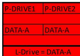
**RAID5:** RAID5 is a stripe with Fault Tolerance, which attempts to bridge the gap between speed and redundancy. This level will always reserve a capacity equivalent to one drive for fault tolerance, regardless of the overall capacity. This means that if you
