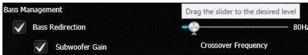
The last section is “Bass Management.” Clicking on “Bass Redirection” enables the Crossover Frequency slider to balance what goes to the subwoofer and satellites. This setting generally will not provide much benefit to headphones, because the bass redirection occurs inside the headphone through its own crossover filters.
