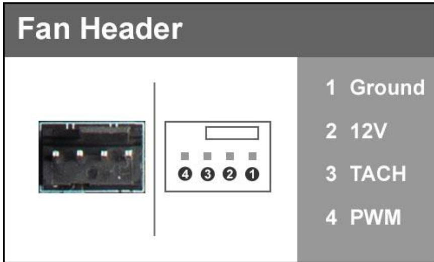
This motherboard line only features 4-pin fan headers, which are backwards compatible with 3-pin fan connectors. The CPU1 and CPU2 fan headers control fans via PWM. The remaining headers control fans by either PWM or DC controls. The headers have an absolute safe power limit of 2 Amp @ 12 Volts (24 Watts). These headers are for your CPU heatsink and chassis cooling fans.
