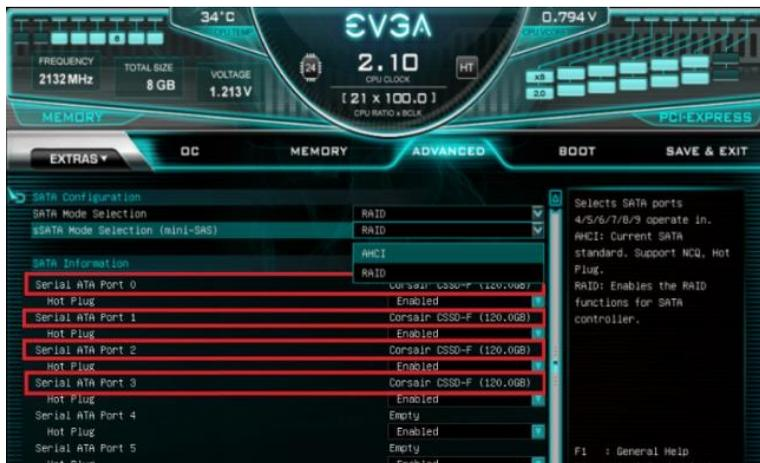
Once RAID is enabled and all devices are detected, press F10 to save and exit. Upon reboot, repeatedly press “Delete” to reenter the BIOS. Once in the BIOS, go back to the “Advanced” tab where you’ll find new items at the bottom of the list called “Intel® VROC sSATA Controller” and “Intel® VROC SATA Controller.”
