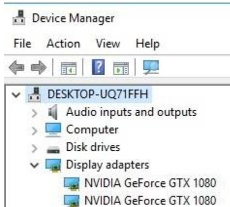
3. Once you have verified there are no detection/driver installation issues with the cards, you can enable SLI. Right-click on the desktop and select “NVIDIA Control Panel” (“NCP”).
