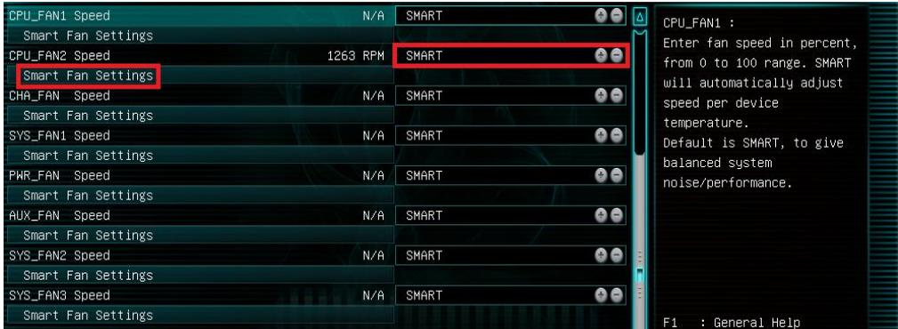
The +/- buttons next to Smart allow you to set your fans at a static speed percentage, instead of a curve. If you set the speed too low, however, the fan may stall; the stall speed will vary from fan to fan.
