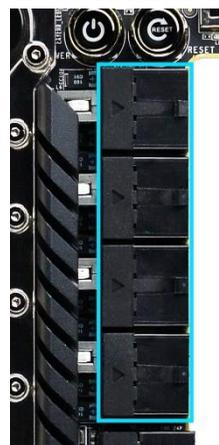
Make sure the plug is fully-seated and also make sure that the tab on the socket and the release on the power connector are on the same side (see the box in **BLUE** on the second picture for the tab on the EPS connector). If the connectors do not line up, then you have plugged in a PCIe 8-pin into the EPS connector, which may cause irreparable damage to the motherboard or the CPU.
