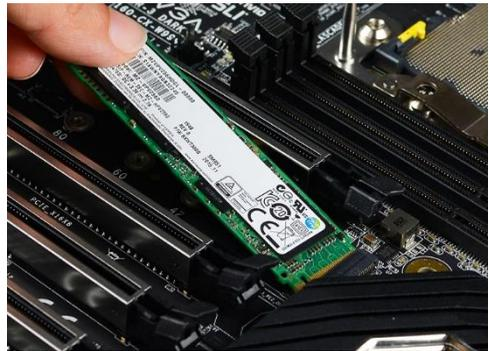
4. Gently push the M.2 device down on the raised end. There will be some tension - this is normal - then use the screw you removed in Step 1 to secure the device. At right, you can see that the contacts will be nearly invisible when the device is properly seated and the copper mounting semi-circle is partially visible around the screw.
