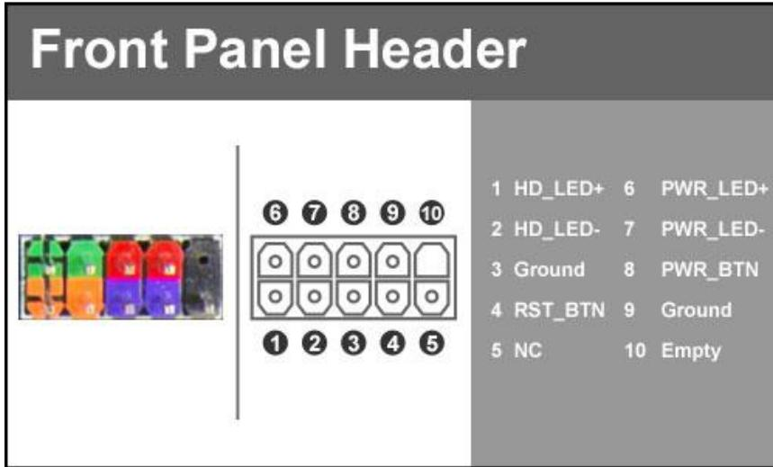
The front panel header on this motherboard is used to connect the following four cables:
