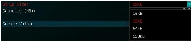
The controller defaults the capacity to the maximum available space for the RAID. Leaving the capacity at default is recommended because reducing the size is not beneficial, except in limited cases.
