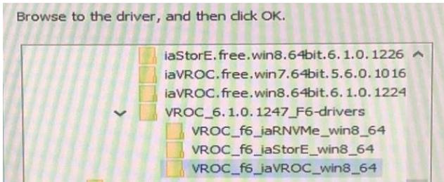
Select the VROC\_f6\_iaVROC driver, as shown above. The OS should recognize the array properly and you should be able to continue your installation.
