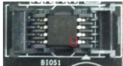
3. Remove the BIOS chip by lifting it straight up. Set it aside and insert the replacement chip. Once installed, close the left door first and the right door second, making sure both latch into place; you will feel a click when this happens. It is normal if the chip moves a little in the socket when closing the left door. Lastly, close the right door. Once both doors are closed, you've successfully replaced the BIOS chip.
