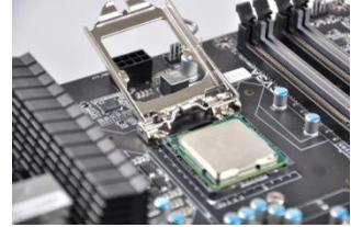
Align notches with notches on the CPU
