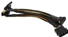
Allows a Molex power connector to adapt to a SATA power connector.
