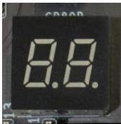
Debug LED with CPU Temperature Monitor
