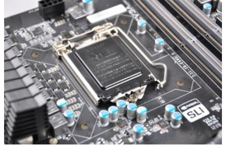
Unhook the socket lever by pushing *down* and *away* from the socket.
