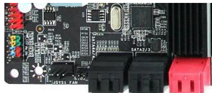
SATA 4a (bottom) SATA 2 (bottom) SATA 0 (bottom) SATA 4b (top) SATA 3 (top) SATA 1 (top)
