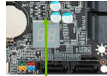
Debug LED with CPU Temperature Monitor
