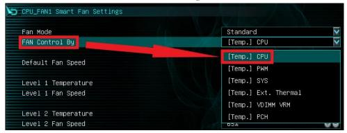
First, choose the temperature monitor the PWM controller will use to monitor for its temp information. It's recommended to link the fan control to the CPU, which is predominantly the most important temperature in the system. The exception is when you have 128GB of heavily overclocked RAM, which may cause PWM temps to be a concern. If this is a concern, set the fan control to the PWM temp.
