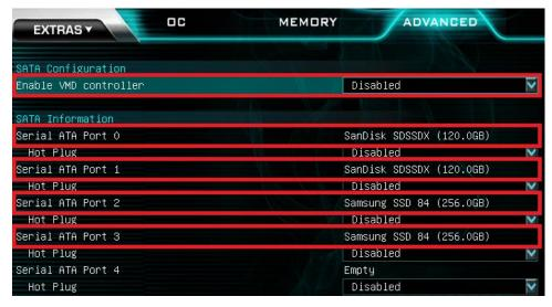
3. Similar to the M.2 RAID instructions, set Enable VMD Controller to "Enabled", then Save and Reboot. Upon entering the menu again, you will notice that your SATA port information will be empty. This mode includes both the RAID controls and the same options/functions/commands as AHCI. As a result, you may continue to use your AHCI devices normally while configuring a RAID.
