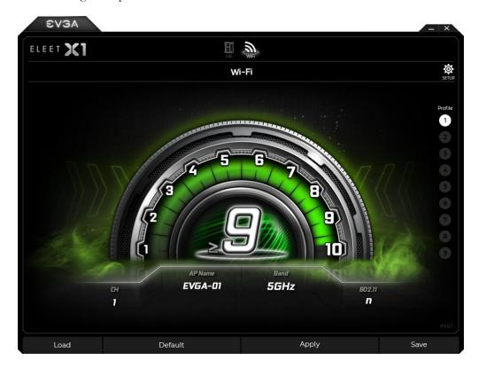
The Wi-Fi page will display typical information about your wireless connection and your signal strength, including your Access Point name, wireless band, and wireless version. The signal strength is indicated on a 1-10 scale, with 1 being the weakest and 10 being the strongest.
