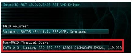
Note: Although any drive that features sufficient capacity will be permitted to rebuild the array, it is recommended to use an exact match or same capacity/performance of the failed drive. The BIOS will remind you, but it cannot be overstated that using a drive with data on it will result in the total loss of all previous data in favor of the data on the array.
