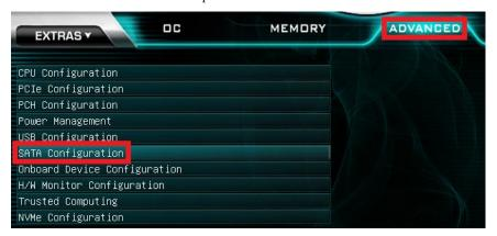
Note: The SATA Configuration menu shows a list of all drives currently detected by the controller. Make sure the list in your BIOS matches what you have plugged in. If it does not, reseat cables on the device(s) in question. If the issue persists, please check the troubleshooting section on Page 104.
