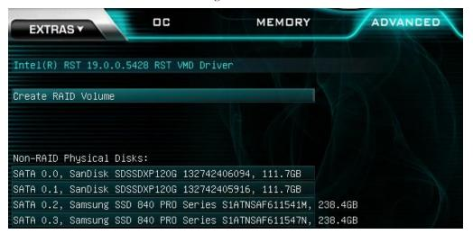
3. The RAID Level is set by default to RAID0 (Stripe), so you will need to change it to RAID5 (Parity). Available drives for the RAID will be listed here, along with a blank box to allow you to select whether you want each drive to be part of the RAID. In this case, we will select all SSDs for the RAID, so we will select each drop-down and choose the "X" option. After configuring your RAID Level, disks, Strip Size, and RAID capacity, select "Create Volume".
