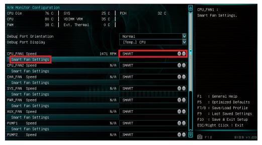
Once into the H/W Monitor section, you can see the temperature monitors across the top. Below the monitors, each fan is already configured in Smart mode, which means the fan controller is using a Smart curve for fan controls. Each fan can be set to a separate fan curve. To set a Smart curve, please see the guide starting at the top of the next page.
