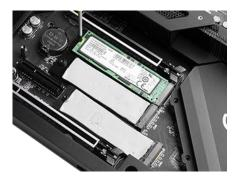
Please carefully check your M.2 devices for proper installation before moving on to the next step. If the M.2 device is not installed properly, the heatsink covers cannot be fully fastened.
