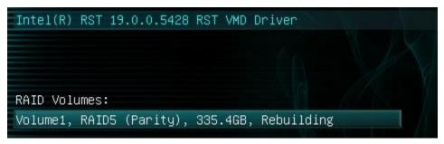
Note: Completing this process in the BIOS queues the rebuilding of the array, but does not start the process until after you restart and boot into your OS. The rebuilding duration will vary – fast drives in uncomplicated arrays can rebuild very quickly, while complicated arrays with redundancy may take several hours to rebuild. The duration of the rebuild process can also be impacted by the usage of the array and system performance during the process.
