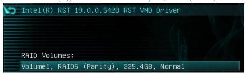
13. For OS installation, provided that the array is configured properly, the operating system will detect the array and see it as a single drive or a bootable RAID array – as opposed to several drives – and allow you to install the OS to the array without any further steps. However, depending on the OS version, you may need to install RAID drivers for the RAID array to be detected.
