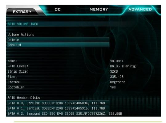
Note: RAID0, RAID1, RAID5, and RAID10 are supported on the Z790 CLASSIFIED when spanned between the M.2 slots and SATA ports, but this is strongly not recommended due to the significant difference in performance and the lack of device uniformity (i.e. different SSDs within the same RAID), which may cause a RAID to become unrecognized or fail unexpectedly.
