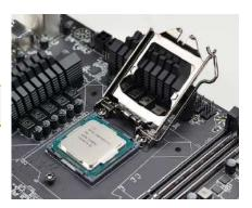
4. Lower the load plate so that it is resting on the CPU.
