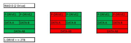
As RAID0 has no fault tolerance, even a single drive failure compromises the array and renders the array Failed and unrecoverable.
