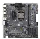
The EVGA Z370 Micro ATX Motherboard This motherboard contains the Intel® Z370 chipset,
