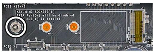
2. Insert the M.2 device at a slight angle - approximately 45 degrees to the board. This will allow the contacts (colloquially called "Gold Fingers") to seat completely into the slot. If the device is fully seated, you should be able to release it and the device will rest at an angle of about 30 degrees on its own, as shown in the picture below.
