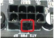
from your PSU manufacturer for your specific PSU, because using a cable designed for a different PSU may have catastrophic effects. Finally, ensure that the cable on the PSU side is plugged into the connector for the CPU, typically labelled "CPU" or "EPS," but consult your power supply manual for the correct plug.
