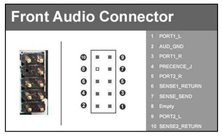
Front panel audio connectors support different audio standards and can provide two kinds of audio output choices: HD Audio, or AC'97 to accommodate older cases that still use AC'97, rather than HD. The Z370 Micro only has a HD Audio front panel connector.
