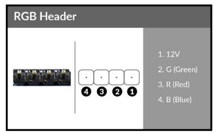
This header and pinout is also shared with the RGB LED header, which also supports 1 Amp @ 12 Volts (12 Watts). This will add control options through EleetX for controlling RGB LED's.
