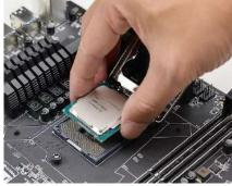
Note: Make sure the CPU is fully seated and level in the socket.
