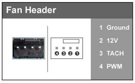
This motherboard line only has 4-pin PWM fan headers, which are backwards compatible with 3-pin fan connectors. Fans may be controlled by PWM or DC controls. The headers have an absolute safe power limit of 1 Amp @ 12 Volts (12 Watts). These headers are for your CPU heatsink and chassis cooling fans.
