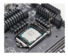
5. Carefully lock the right lever back into place by lowering it down to the hook, then push the lever towards the socket and down under the hook.
