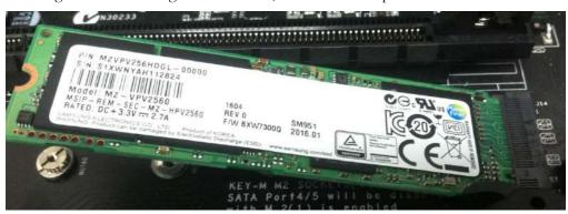
3. Gently push the M.2 device down on the raised end. There will be some tension - this is normal - then use the screw you removed in Step 1 to secure the device. Below, you can see that the contacts will be nearly invisible when the device is properly seated and the copper mounting semi-circle is partially visible around the screw.
