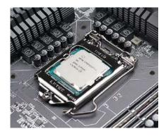
6. Remove the plastic protective socket cover by pulling it straight up and away from the socket.
