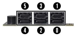
SATA ports on this platform natively support full AHCI and RAID functions. AHCI is enabled by default, but the controller can be put into RAID mode in the BIOS. RAID mode supports RAID levels 0, 1, 5, and 10 through the Intel® controller, and all ports retain full AHCI functionality in RAID mode.
