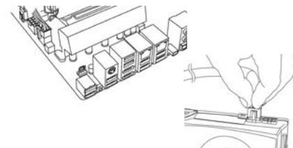
5. Connect the SATA cables to your power supply and drives (hard drives, solid state drives, optical drives).
