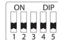
DIP Switch #5 must be turned on for other Dip Switches to operate. While DIP Switch #5 is on, the DIP switch settings will take priority over firmware or software settings. While DIP Switch #5 is turned off, the PSU will default to the settings present in the PSU firmware or in the SuperNova software.
