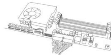
4. Connect the 8-pin EPS12V cable(s) to the power supply and the motherboard. Connect the 6/8-pin PCIe cables to the power supply and your graphics card(s). **NOTE:** Do not attempt to plug an 8-pin PCIe cable into a 6-pin connector without first detaching the two extra pins.
