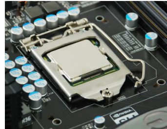
Align notches with notches on the CPU
