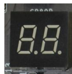
Debug LED with CPU Temperature Monitor
