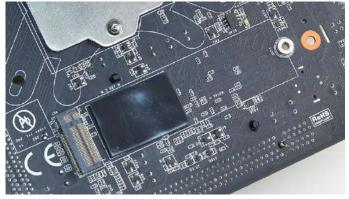
3. Insert the M.2 device at a slight angle of approximately 45 degrees to the board. This will allow the contacts (colloquially called "Gold Fingers") to seat completely into the slot. If the device is fully seated, you should be able to release it and the device will rest at an angle of about 30 degrees on its own, as shown in the picture to the right.
