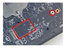
2. After adding the thermal pad, the motherboard will look like the image below. This thermal pad will assist with cooling your M.2 Key-M device.
