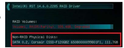
Select the degraded RAID volume, then select "Rebuild" on the following menu.
