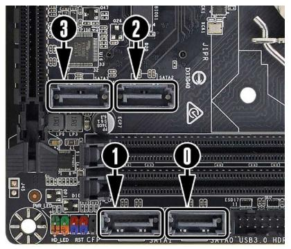
SATA ports on this platform natively support full AHCI and RAID functions. AHCI is enabled by default, but the controller can be put into RAID mode in the BIOS. RAID mode supports RAID levels 0, 1, 5, and 10 through the Intel<sup>®</sup> controller. RAID-ready ports also have full AHCI functionality.
