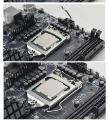
Note: After removing the CPU socket cover, it is recommended to store it in case you ever need to transport your motherboard. If you ever remove the CPU, it is highly recommended to reinstall the socket cover.
