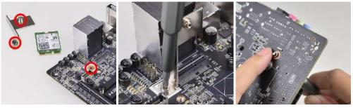
2. (Left) Insert your M.2 Key-E device into the slot. (Middle) Secure the device with the screw you removed in (Left), until fully tightened (Right).
