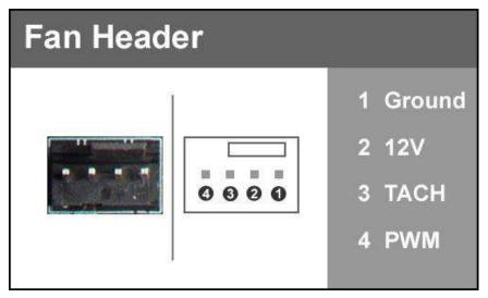
This motherboard line only has 4-pin fan headers, which are backwards compatible with 3-pin fan connectors. Fans are controlled via PWM controls. The headers have an absolute safe power limit of 1 Amp @ 12 Volts (12 Watts). These headers are for your CPU heatsink and chassis cooling fans.
