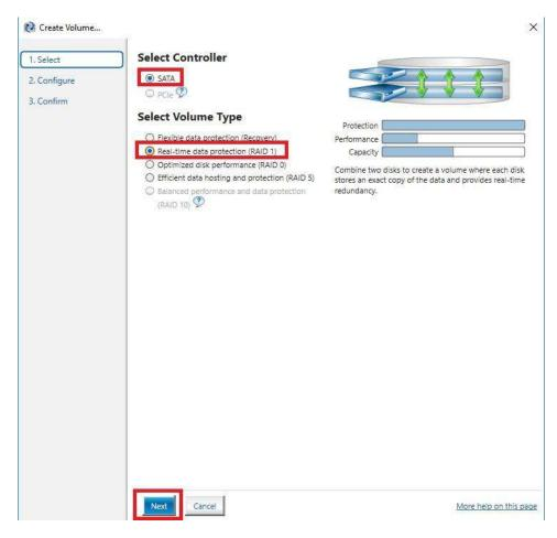
SATA will be selected by default. PCIe primarily refers to PCIe / M.2 based NVMe drives; the same basic steps do apply to both, however. Select SATA, and "Real-time protection (RAID1)." Then, click Next at the bottom of the window.
