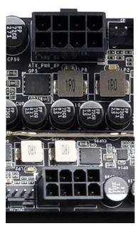
Also, only use cables from your PSU manufacturer for your specific PSU, because using a cable designed for a different PSU may have catastrophic effects. Finally, ensure that the cable on the PSU side is plugged into the connector for the CPU, typically labelled "CPU" or "EPS," but consult your power supply manual for the correct plug.
