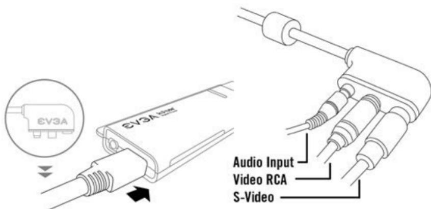
1. Connect the AV-input adapter (included) into the input located on the rear of inDtube next to the gold plated MCX input. The AV-input on inDtube is notched and will only fit one way. Do not force in as this may cause irreversible damage to both the AV-input adapter and inDtube.
