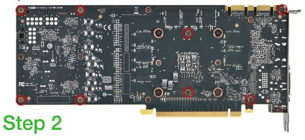
Remove the protective cover from the backplate. Place on back of card and align the screw holes.
