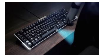
EVGA Time-of-Flight Sensing System The Z20 keyboard features a ToF proximity sensor, this detects user movement to trigger the system awake or to send it to sleep.
