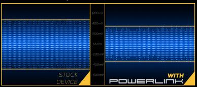
The 12V line going into graphics card without a PowerLink™ under load rates a Peak-to-Peak voltage of 1,008mV, while the 12V line going into the graphics card with a PowerLink™ is only 728mV. That's nearly a 28% reduction in voltage variation from the external power source!
