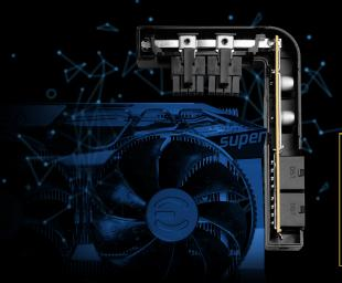
The PowerLink™ features two solid state capacitors that help to filter/suppress ripple and noise from the power supply.
