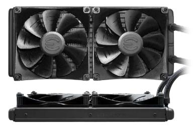
The EVGA CLC 240 LIQUID CPU Cooler has arrived! This new liquid cooler from EVGA gives you incredible performance, low noise, and robust software controls. The full copper waterblock pulls the heat from your CPU to the radiator, where newly designed fans, featuring Teflon Nano Bearings, effortlessly disperse the heat.
