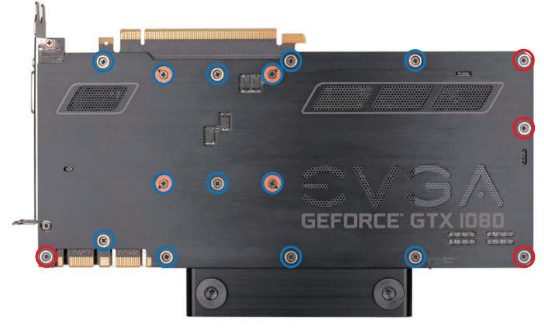
8) Installation is now complete. Ensure that the PCB is not bent (if it is, you have over-tightened some of the screws). It is recommended to check during testing whether the nameplate LED lights up when you turn on the PC. If it does not, then you may need to remove the waterblock to check the connection.
