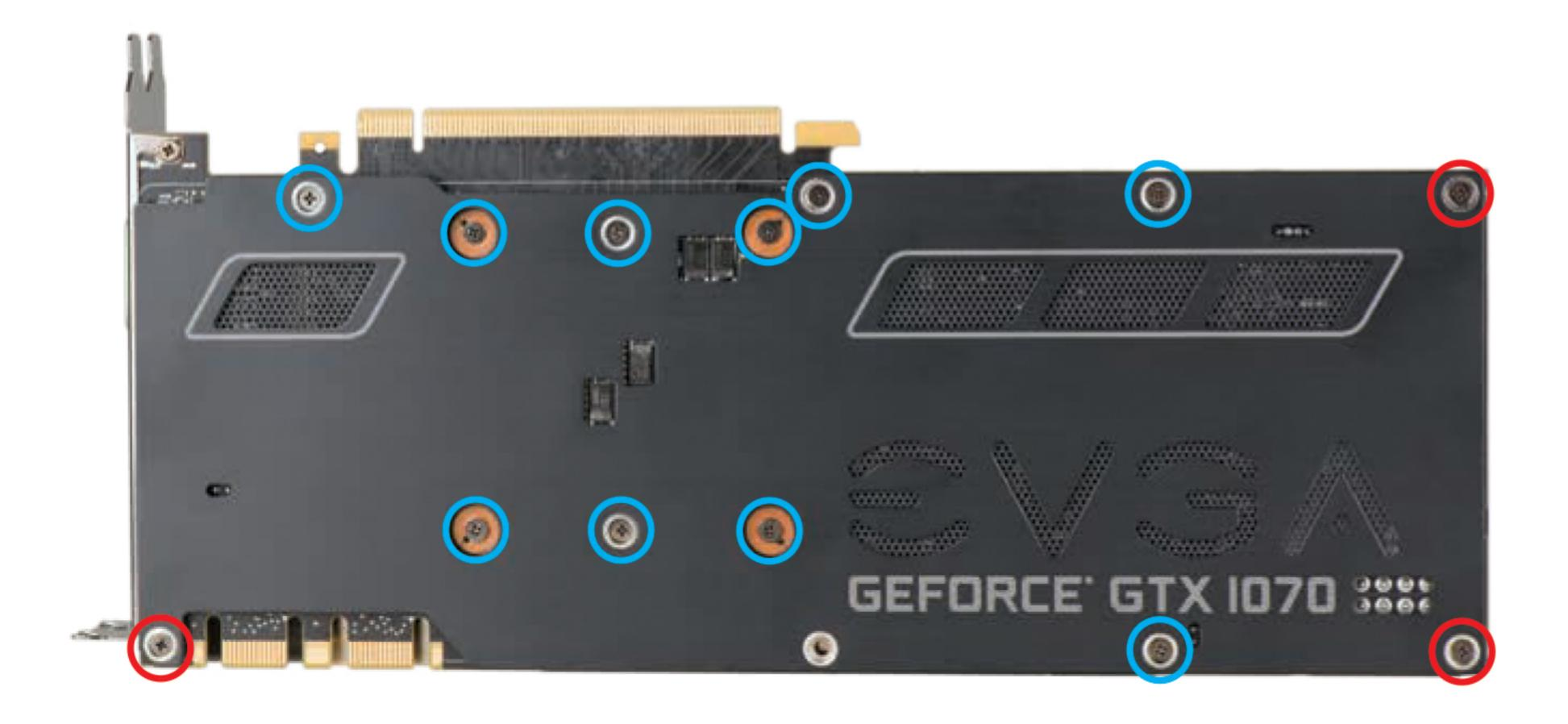
B3. Installation is complete, ensure that the PCB is not bent (if it is you have over-tightened some of the screws) the LED on the nameplate should be on when the PC is powered, and ensure all 6 ports on the connection block are sealed, with either some type of connection or a plug.
