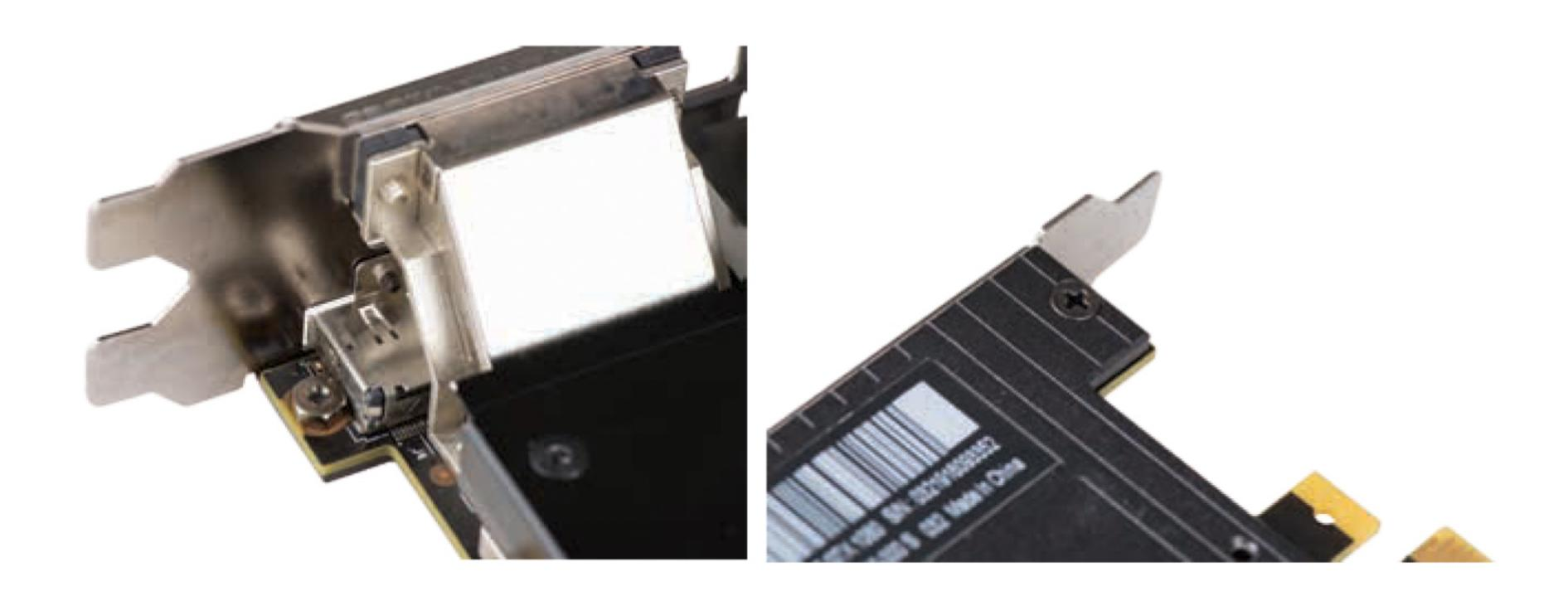
A4. Installation is complete, ensure that the PCB is not bent (if it is you have over-tightened some of the screws) the LED on the nameplate should be on when the PC is powered, and ensure all 6 ports on the connection block are sealed, with either some type of connection or a plug.
