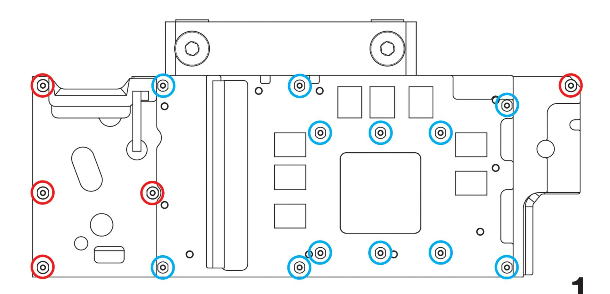
1) Remove the all screws and 4 spring screws on the back side of the card as well as the 2 on the bracket, (if you are using Founders Edition Card).
