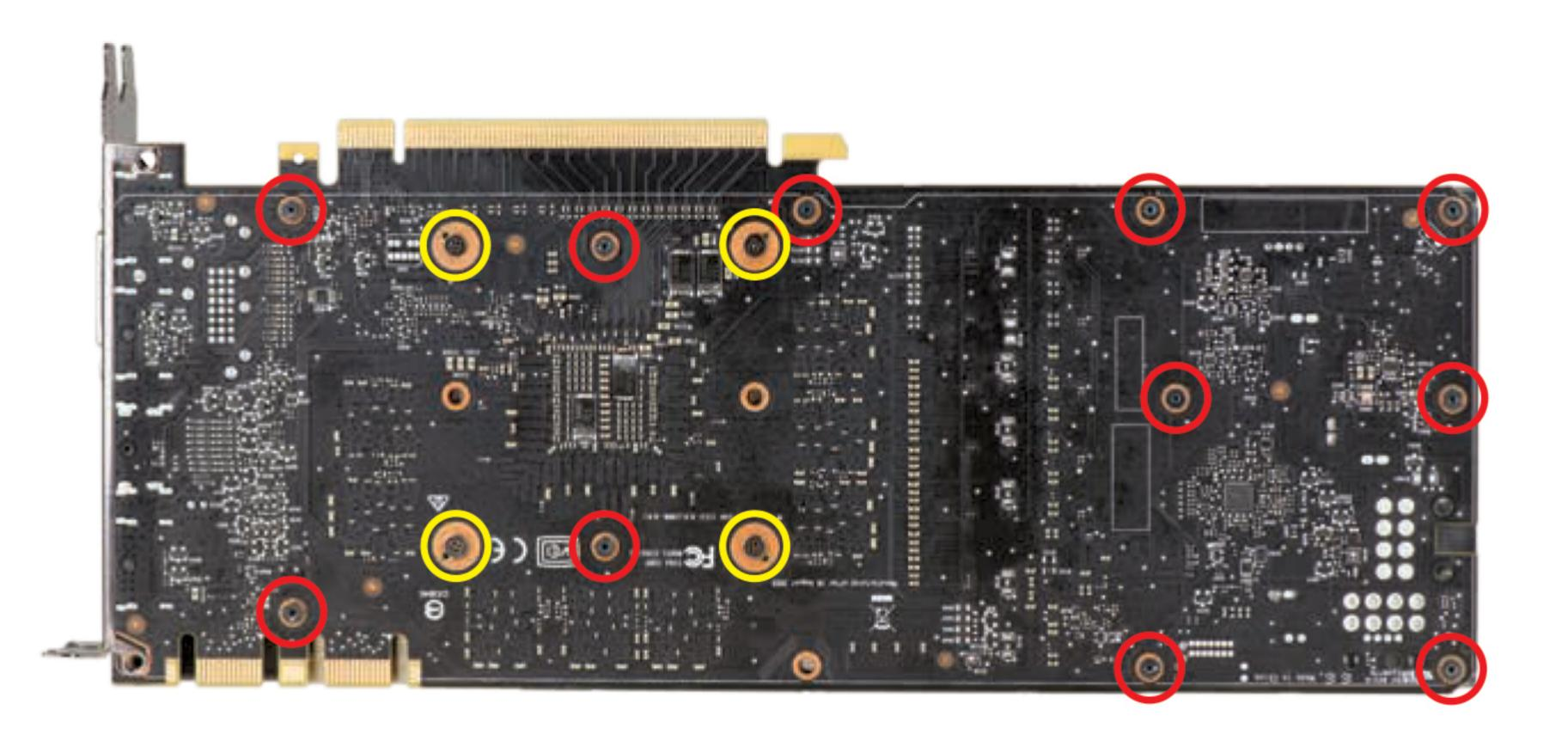
A2. Finish aligning waterblock and install the 11 pcs original small screws into the backplate.
