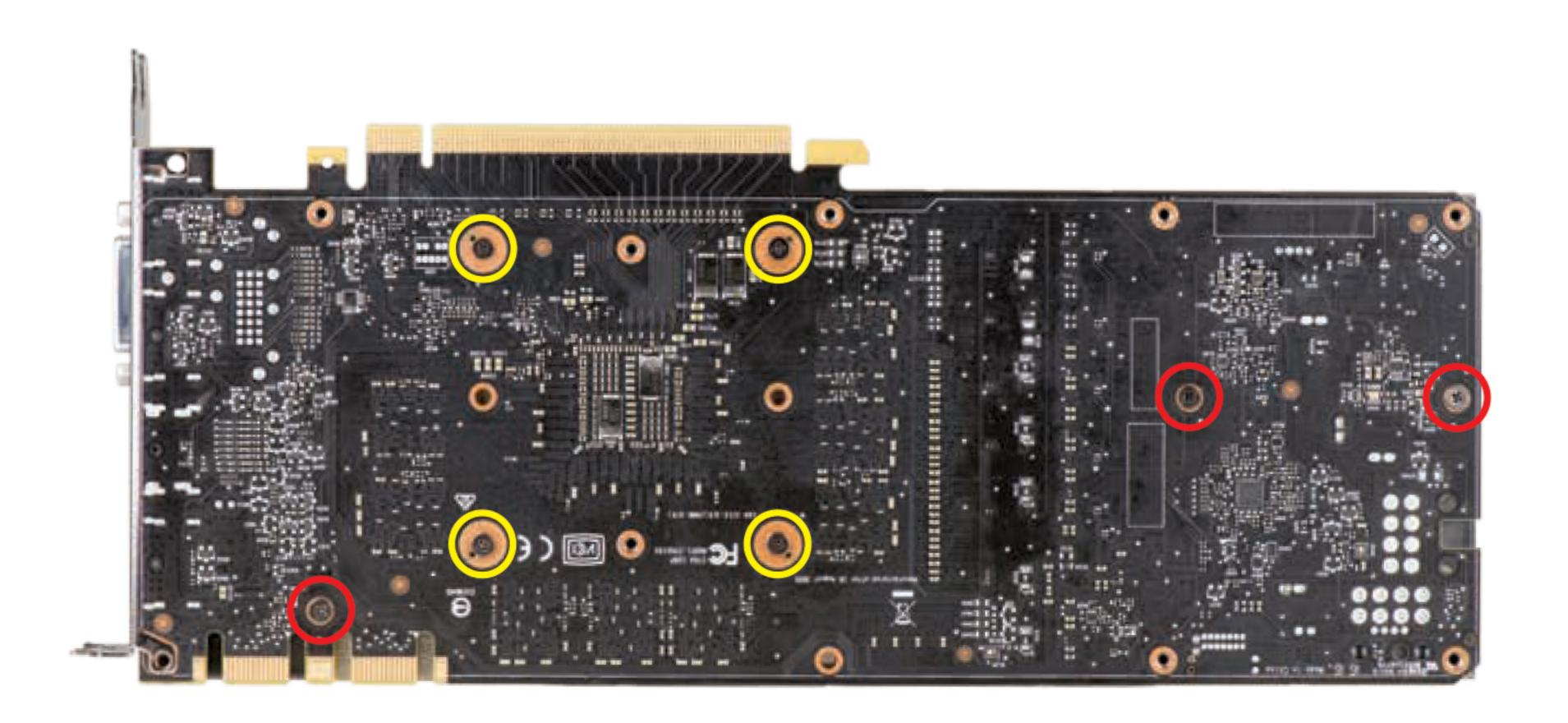
B2. Place backplate on card then screw up all. The red circle use long screws and blue use short screws.
