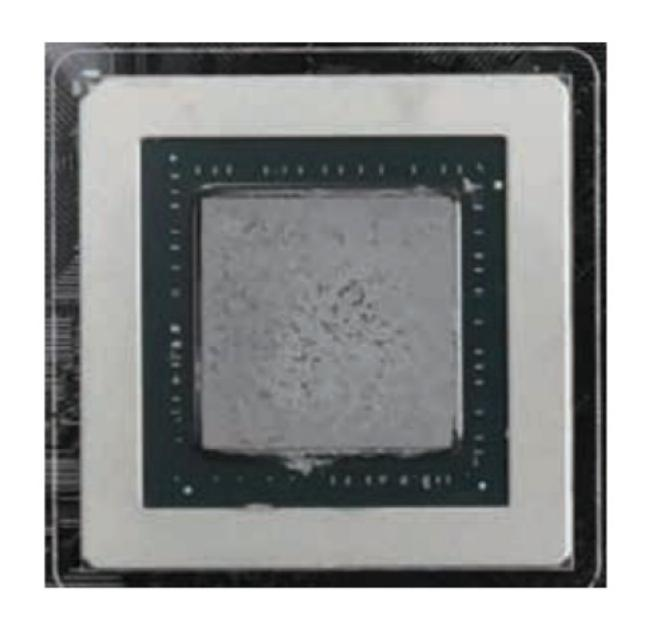
4) Remove protect film on Thermal Pad of waterblock, then install the waterblock on the card of
