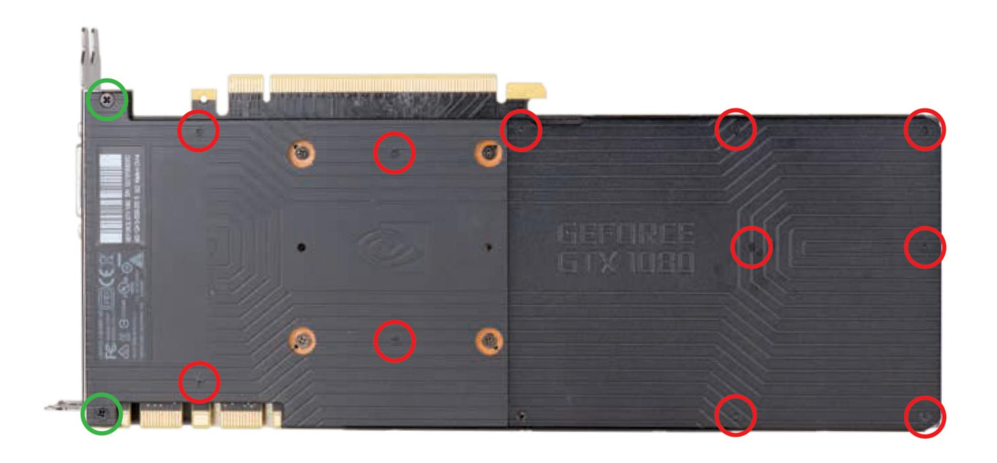
A3. This screw holds down the bracket and needs a nut on the back to hold it in position.
