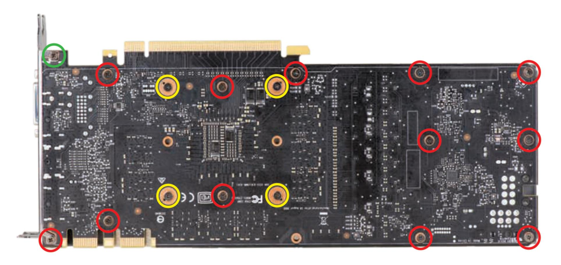
C2. Installation is complete, ensure that the PCB is not bent (if it is you have over-tightened some of the screws) the LED on the nameplate should be on when the PC is powered, and ensure all 6 ports on the connection block are sealed, with either some type of connection or a plug.
