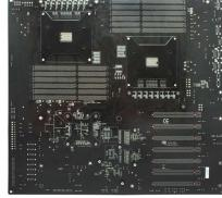
Supported CPU's - Intel® Xeon® Dual QPI Processors Socket Type - 2 x LGA1366 QPI - Up to 6.4GT/s
