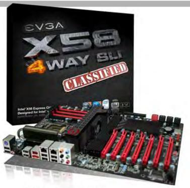
EVGA X58 4-Way SLI Classified is in a league of it's own. Featuring an incredible seven PCI Express Graphics Expansion slots, which enables support for the World's First 4-Way SLI Graphics card, the EVGA GTX 285 Classified.
