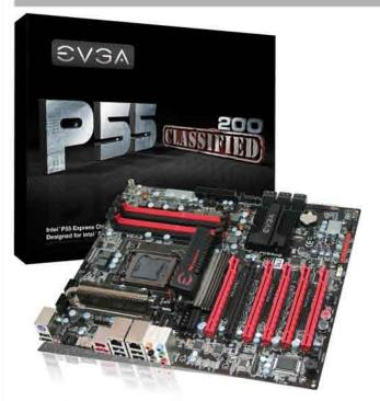
EVGA P55 Classified 200 motherboard features the latest Intel P55 Express chipset support Socket 1156 based processors. With support of up to eight threads of computing power, dual-channel DDR3 memory at frequencies of 2600MHz and beyond, NVIDIA 3-Way SLI Technology, EVGA Show-Volt and much more, the EVGA P55 Classified 200 offers enthusiast level performance, features and overclocking.
