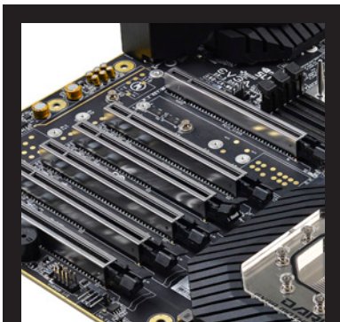
REINFORCED PCIe SLOTS Reinforced for the heaviest of graphics cards
