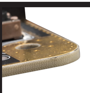
16 LAYER PCB Improved overclock stability and PCB cooling
