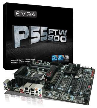
EVGA P55 FTW 200 motherboard features the latest Intel P55 Express chipset supporting Socket 1156 based processors. With support of up to eight threads of computing power, dual-channel DDR3 memory at frequencies of 2600MHz and beyond, and NVIDIA 3-Way SLI Technology, the EVGA P55 FTW 200 offers enthusiast level performance, features and overclocking!
