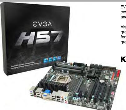
EVGA H57 motherboards feature the Intel H57 Express chipset supporting Socket 1156 based processors. This motherboard is engineered to be the ultimate media platform with support for DVI, VGA and DisplayPort right on the board, an external graphics card is not necessary.
