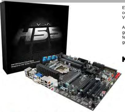
EVGA H55 motherboards feature the Intel H55 Express chipset supporting Socket 1156 based processors. This motherboard is engineered to be the ultimate media platform. With support for DVI, VGA and DisplayPort right on the board, an external graphics card is not necessary.
