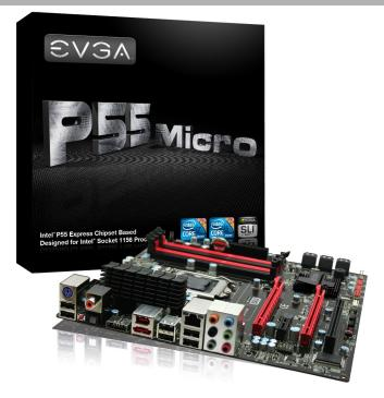
EVGA P55 Micro motherboard features the latest Intel P55 Express chipset supporting Socket 1156 based processors. With support of up to eight threads of computing power, dual-channel DDR3 memory at frequencies of 2000MHz and beyond, NVIDIA SLI Ready, EVGA Dual Play Heatsink support and more, the EVGA P55 offers great features at a great price!
