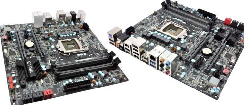
Supported CPUs - Sandy Bridge 2<sup>nd</sup> Generation Intel® Core™ i3, Core™ i5 and Core™ i7 Socket 1155 Socket Type - LGA1155
