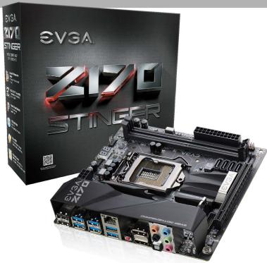
The EVGA Z170 Stinger motherboard is engineered to exceed the best. Featuring a next generation Intel Z170 Express Chipset with DDR4 3200MHz+ memory support, this motherboard is built to perform. Four native SATA 6G ports, eight native USB 3.0 provide robust storage and I/O options, and the mITX form factor allows for an extremely compact performance system.
