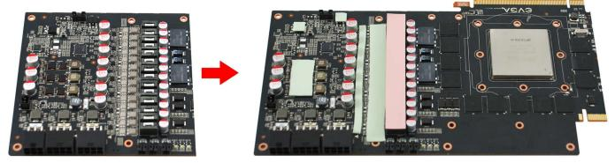
Step 3 Place black heatsink on the rear of the card and the GPU riser around the GPU.
