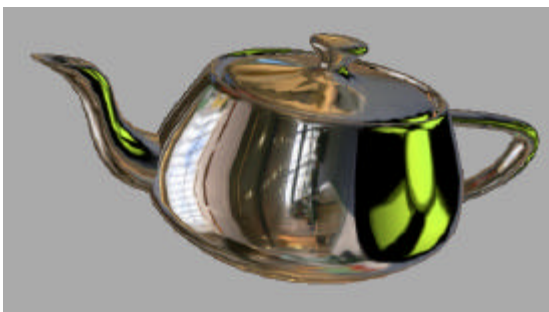
A cube environment map is applied to this teapot. The texture coordinates needed to apply the cube map to the teapot were generated with a Vertex Shader.
