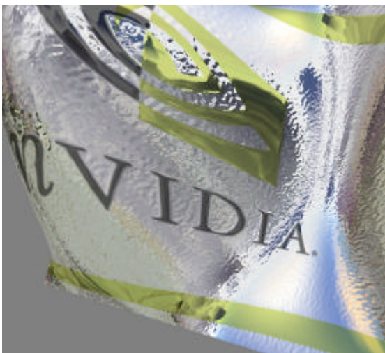
Using programmable Pixel Shaders, it's now possible to implement shiny bump maps that look correct from all angles and do not distort as the angle of lighting varies.
