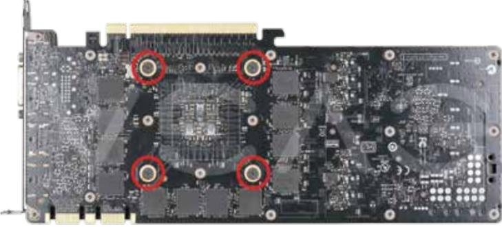
3) Remove the 4 spring screws on the back side of the card (#1 Phillips Bit) this will allow the heatsink to be removed.
