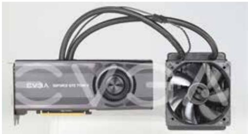
The EVGA GTX™ TITAN X Hybrid Kit is exclusive only to the NVIDIA® Reference PCB/Air cooling GTX™ TITAN X graphics card and was not designed to fit on any other graphics card.
