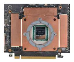
(b) Please check to make sure that your thermal pads are in the same location as photo below. If not, please check the back of the card in case the matching thermal pad remains on the card. Install the memory baseplate, as shown in Step 4(a). Hold the copper plate in place and turn the card over. Place the right backplate over the card and tighten the backplate with 4 #8 screws, as shown in the left photo below.
