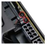
(c) Install the shroud over the PCB. Make sure to slide the shroud under the edge of the PCI bracket, as shown in the left photo below. Once the shroud is in place, tighten 2 #7 screws in the area circled in red, as shown in the right image below.
