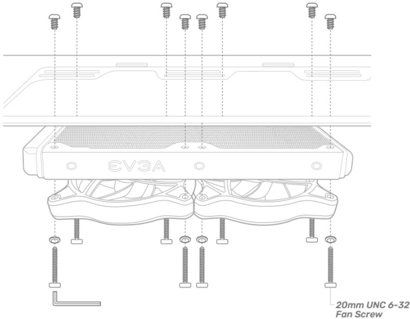
**Warning** – The CLCx Cooler is not a passive cooler. Fans must be installed to the radiator for proper operation of the CLCx Cooler, and failure to do so may cause irreparable damage to the pump and other connected hardware.
