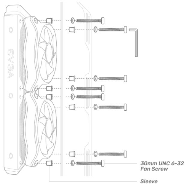
**Warning** – The CLCx Cooler is not a passive cooler. Fans must be installed to the radiator for proper operation of the CLCx Cooler, and failure to do so may cause irreparable damage to the pump and other connected hardware.
