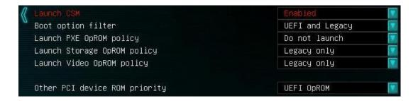
Storage option ROM need to be enabled to allow usage of external storage/RAID controllers, such as PCIe SAS cards.
