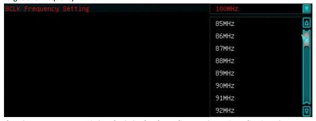
The BCLK Frequency range is 85 Mhz-250 Mhz, depending on BCLK ratio. Adjusting BCLK may not be an ideal way to overclock the system, as it affects all subsystems, like memory, PCI-E, peripherals, however in short order you may start seeing drastic stability issues.
