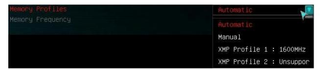
The options are Automatic, Manual, and XMP Profile 1 and 2. Automatic is the default speed set by the BIOS to ensure the system boots initially so correct values can be set. Typically the frequency will be below advertised, and the latency will be higher, this is for universal compatibility.
