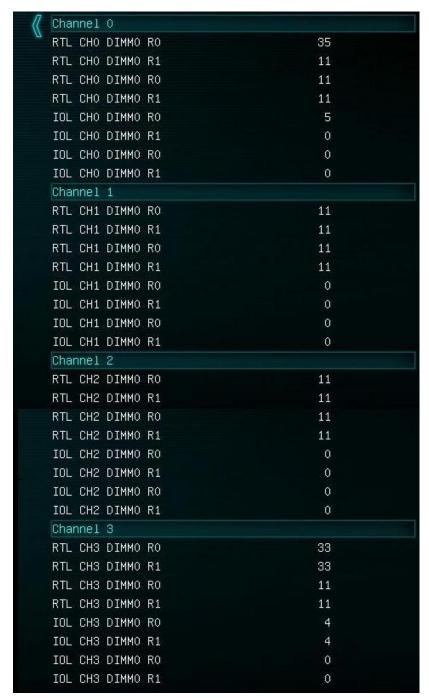
Manual adjustment should not be necessary unless the system is running speeds in excess of 2400 MHz or higher BCLKs where some drift may cause read/write leveling.
