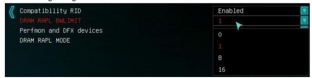
This is a limiter for average power consumption for the DRAM module. (1 is the recommended Intel Value).
