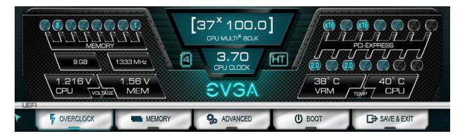
In the center above the EVGA logo, is basic CPU information. There is the overall CPU clock speed shown in GHz (Gigahertz). Above that the CPU Multiplier times Base Clock (BCLK) which is how clock speed is derived. Adjacent to the CPU Clock there is a small outline of a chip and a number inside of it, the number in this case 4, is the number of physical cores in the CPU. HT indicates that Hyper Threading is enabled.
