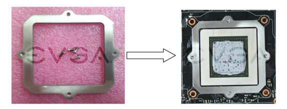
2. Insert 4 screws to secure the bracket.
