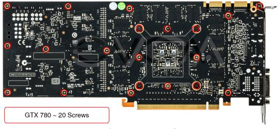
3) Remove all thermal paste and pads from the exposed GPUs and memory. It is recommended to use 91% Isopropyl Alcohol to aid in removing the stock thermal paste. Once you have properly removed the thermal paste from the IHS and the Isopropyl Alcohol has completely dried, add a pea sized drop of the provided thermal paste to the center of the GPUs. Also, peel off the protective film on the included thermal pads.
