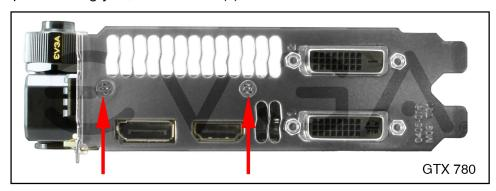
2) Flip the GTX 780 on its back so the fan is facing downwards. Remove all the screws from the underside of the GTX 780 (highlighted below). Now carefully remove the top portion of the heatsink from the GPU. Be careful when removing the shroud as you will need to also disconnect the fan and LEDs.
