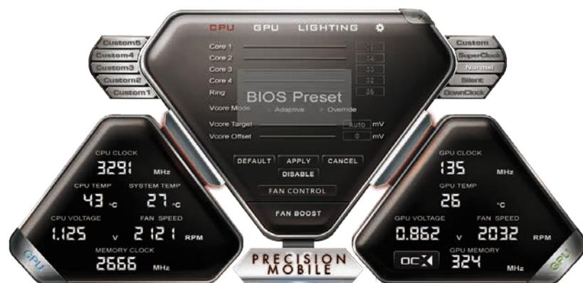
Precision X Mobile is designed to be your monitoring and tuning suite for your EVGA SC17 GEFORCE® GTX 1080 GAMING Notebook. This will cover monitoring in the upper section as well as specific controls for CPU, Motherboard, Graphics card, lighting, and general non-performance/appearance options.
