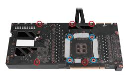
9. Reinstall the I/O bracket and loosely fasten the 3 screws you removed earlier.
