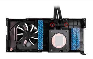
6. Remove the GPU/Memory heatsink from the HYBRID kit and place it over the 4 mounting holes over the pump/waterblock as seen in the image below. At this time, remove any protective covering/tape over the thermal pads before moving to the next step.
