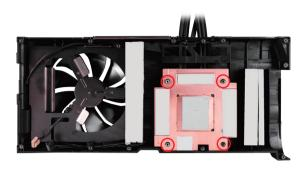
7. At this time, you will install the PCB onto the HYBRID cooler. First, you will need to reconnect the fans and LED connector. Connect the LED connector first, then connect the beige and black fan connectors to their respective headers. The blue header will remain empty. Lastly, line up the screw holes and lower the PCB onto the HYBRID cooler.
